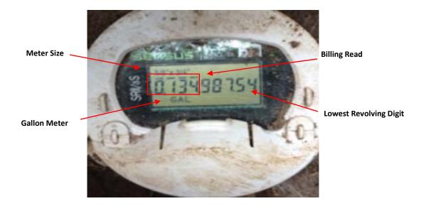
• This is the newest type of meter being installed in our system. The register's lowest revolving dial is to the 1/10 of a gallon. The reading for this register is 34.
