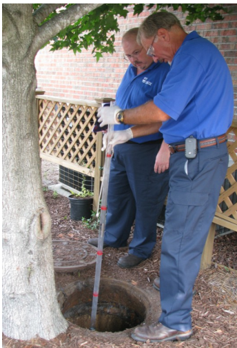
Compliance Officers use a “sludge judge” during an inspection of a local restaurant’s grease interceptor.
